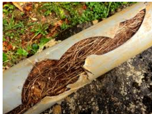
Invading roots can easily invade and destroy pipes.
