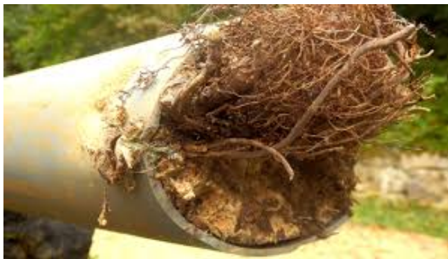
Invading roots can easily invade and destroy pipes.
